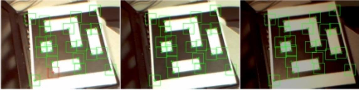
**Figure 5.9 – Continuous corner tracking under lighting changes**
