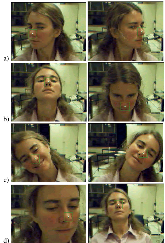
Figure 4: The figure shows the range of motion within which the nose feature is tracked.
