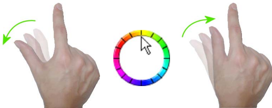
Figure 5.4 - Flicking motion for the ThumbWheel widget. Left flicking decreases a continuous valuator, while right flicking increases the valuator. The speed of the flick controls the granularity of the parameter adjustment. The widget is visualized with a rotating dial.
