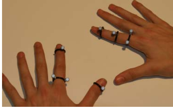
Figure 2.8 – Reflective markers for thumb and index finger tracking [Gros04].
