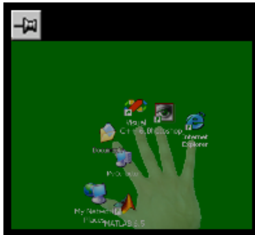
Figure 4.14 – Placing multiply selected objects. The selected icons appear on each finger based on selection order. Tapping a finger releases the icon closest to the tip.
