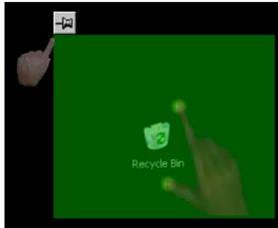
Figure 4.11 – A workspace that can be coarsely positioned using the left hand (shown at top-left of the semi-transparent overlay), while the right hand performs fine manipulations inside of it.
