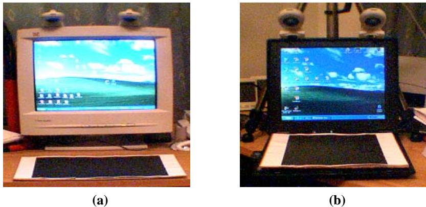
Figure 3.1 – Example configurations for the Visual Touchpad: (a) Desktop; (b) Laptop.
