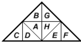
Figure 17 - Rendering order assuming a left-right tree traversal (A = first, B = second, etc.)
